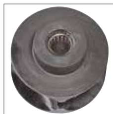
Load chain sheave with needle bearing
