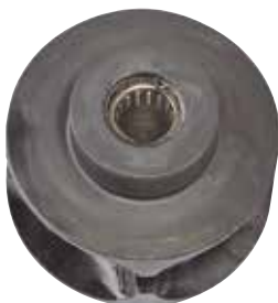
Load chain sheave with needle bearing
