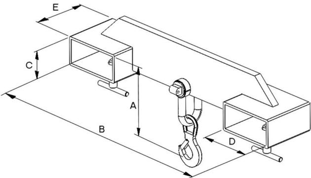
CONTACT Adjustable Fork Mounted Hooks are the most cost effective way of safely hanging a load under the forks of your lift truck. Simply clamps on the forks anywhere along there length.
