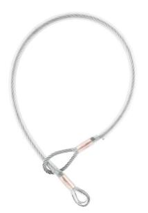
Connecting lanyard AT 191 is a component of personal fall protection equipment. The anchor point should be used as a portable temporary anchor device type B, enabling connection of connecting and absorbing device to a structural anchor point. Connecting lanyard is formed by stainless steel cable, 8mm dia and 0.6 to 10m long, fitted with loops of various diameters at both ends, enabling for looping without using any additional connectors.
