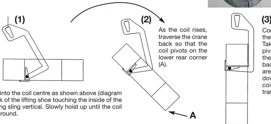
Place the hook into the coil centre as shown above (diagram 1), with the back of the lifting shoe touching the inside of the coil and the lifting sling vertical. Slowly hoist up until the coil rises from the ground.
