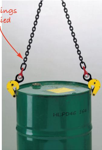
The DC500 drum clamp has been designed to lift and transport steel drums. If moving empty or sealed drums then one clamp is sufficient. Should you be lifting an open full drum, then two clamps should be used with a two leg chain sling.
